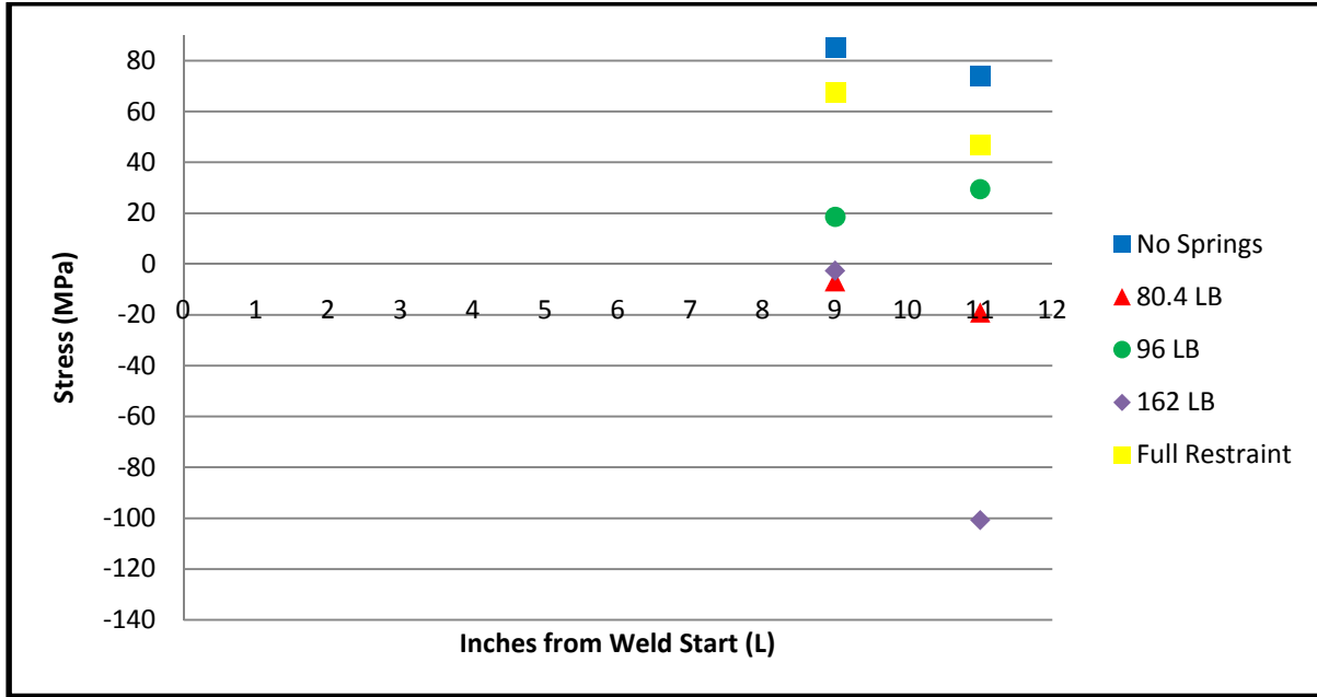
Figure 27. Residual stress data at T = 0.40 for welds performed at John Deere
