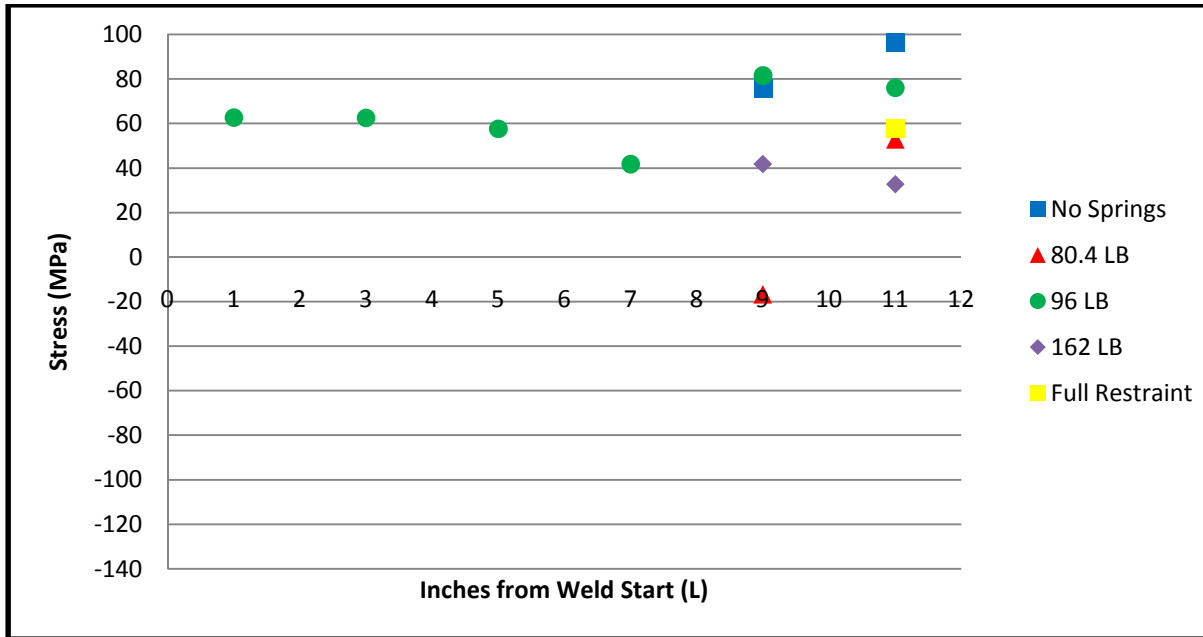
Figure 25. Residual stress data at T = 0 for welds performed at John Deere
